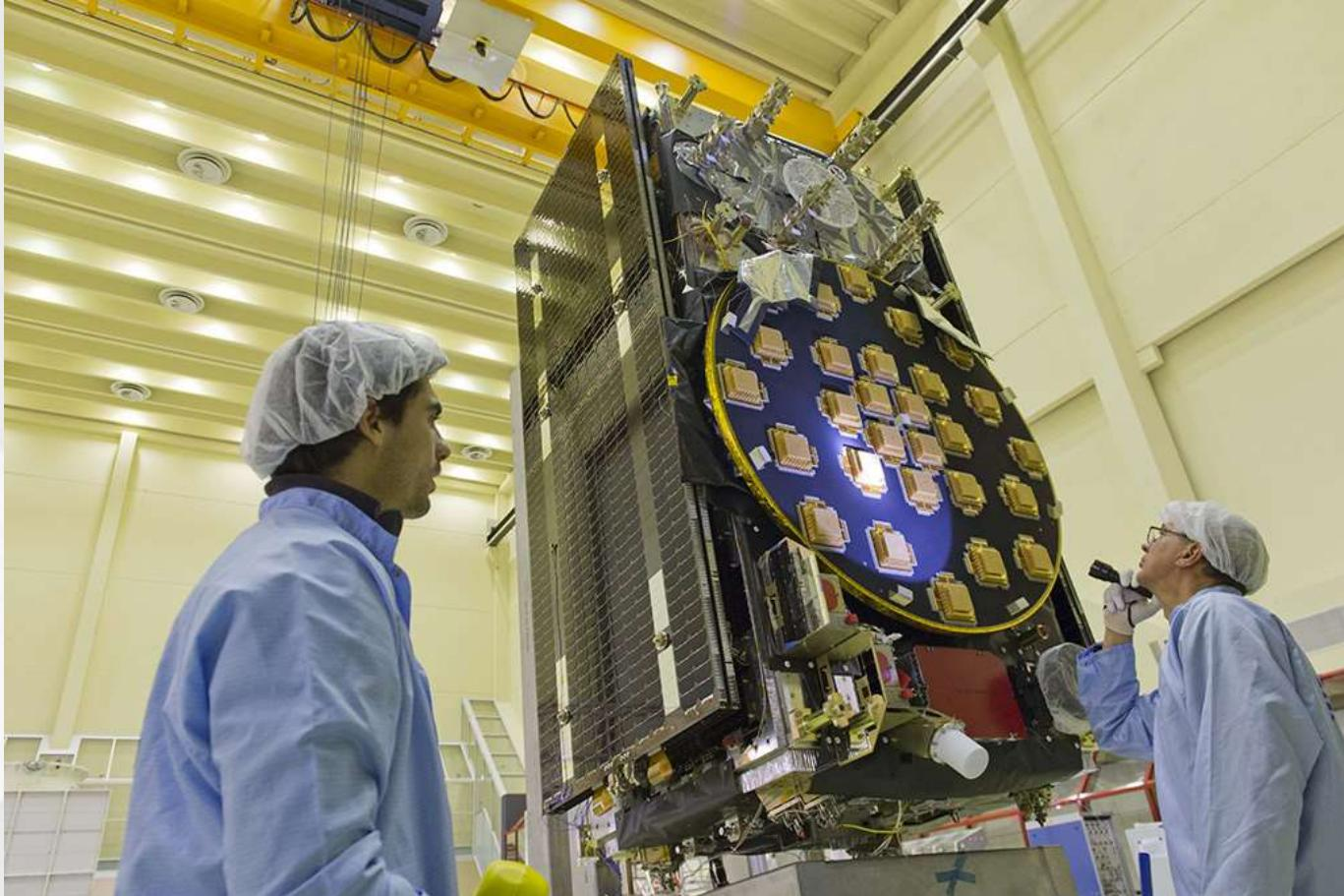
Inspection of main Antenna of 2<sup>nd</sup> Full Operational Capability (FOC) Galileo Satellite
